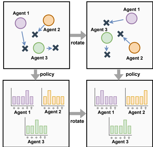
Figure 1: Illustration of multi-agent symmetry. Rotating the state globally in the cooperative navigation task results in a permutation of the optimal joint policy.
